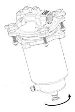
Since there are no moving parts, maintenance is limited to an occasional rinsing of the catalyst core using light fuel oil or detergent. This should be done in accordance with filter changes especially in heavy fuel oil.
